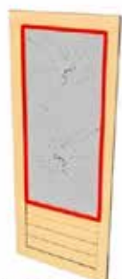
1. Use knife/screwdriver around wooden sticks trim to carefully loosen nails.
