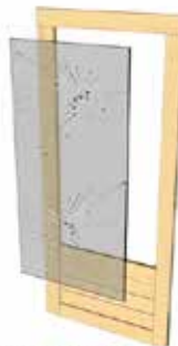
3. Remove broken/damaged glass (if something still holds it, check for leftover nails or cut around glass corners with sharp knife).
