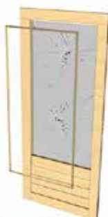
2. Remove trim which holds glass (be careful as it breaks easily).
